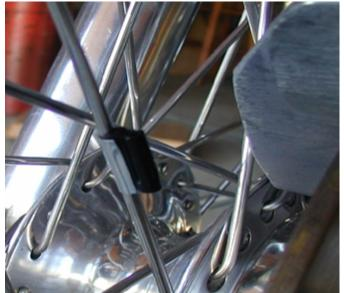
The Magnet attaches directly to the wheel spokes. Since the spokes on a motorcycle wheel are larger than a bicycle you will have to increase the diameter of slot made for the spoke. I held the magnet with a vise, then used 1/4 in drill bit to increase the size. Be careful, you are working with plastic and the heat created by drilling will melt the plastic.
